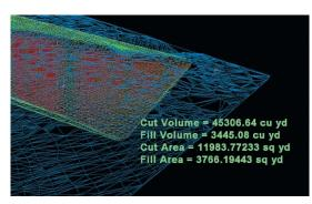
Ground surface TINs and other meshes are easily created and offer great value. Here is an automated report analysing cut and fill quantities using beforeand-after scan data of a ground surface.
