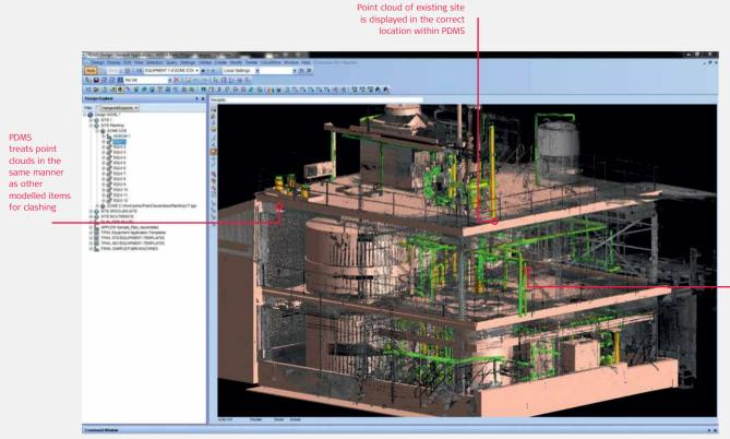
New 3D object exchange for between PDMS and Cyclone
