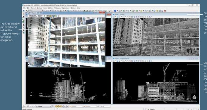
Clear viewing of entire job site with out the need to load only partial jobs. Load rendering of unlimited points using JetStream.
