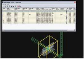
Clash Manager creates a database for managing, tracking, assigning and classifying clashes. A powerful navigation feature lets users easily pull up isolated views of any clash. Here we see a pipe clashing with scanned point cloud data of a beam.
